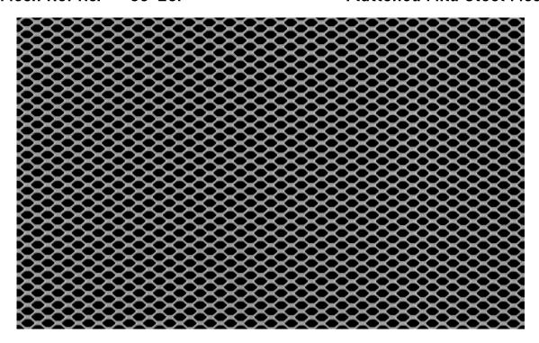
LW Aperture:3.81mmStrand Width:0.79mmSW Aperture:2.03mmThickness:0.60mmWeight:2.11 kg / m2Open Area:56%
